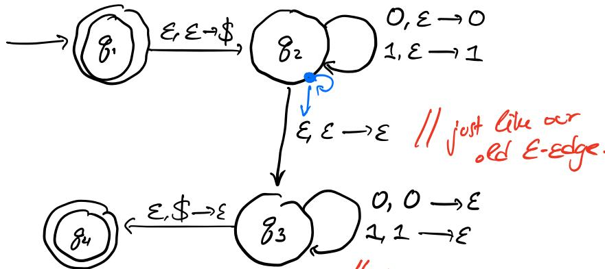
// if in  $q_3$ , read '0' on input and have '1' on stack - die.
