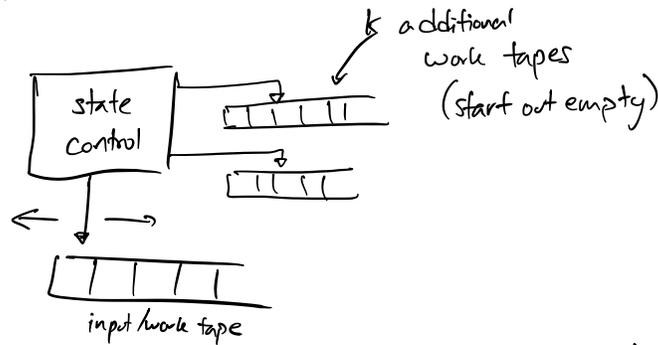
Formally, the Multitape TM is a 7-tuple like the TM but with the transition function
