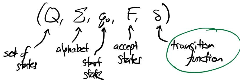
$$\delta: \overbrace{Q}^{\text{a state}} \times \overbrace{(\Sigma \cup \{\epsilon\})}^{\text{character (or } \epsilon \text{)}} \rightarrow \overbrace{\mathcal{P}(Q)}^{\text{a subset of states.}}$$
